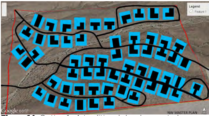
Figure 14: Option 1. A traditional development plan without conservation design, 60 3-acre lots, 87.5% Development' 13% NOS,
